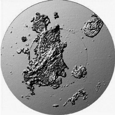
Figure 10. Top: Confocal microscope photo simulation view of end-face contaminated with silver particles. Bottom: Photo simulation view after the fifth mating. Transfer occurred after first mating and now appears to cover the fiber core.
